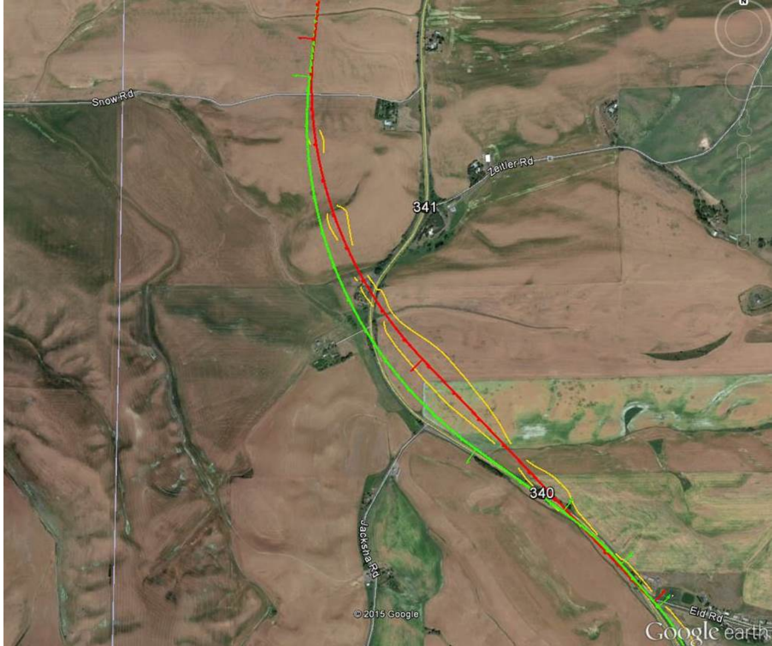
Revised W4 Alignment: Thorn Creek to Moscow Green Line – Original Alignment Red Line – Revised Alignment Yellow Lines – Top of Cut Dimensions
